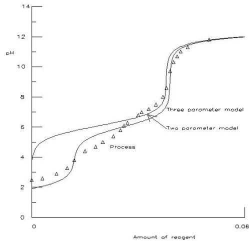
Fig. 13. Titration curves of the process, the two parameter model and the three parameter model in the experiment 2.
