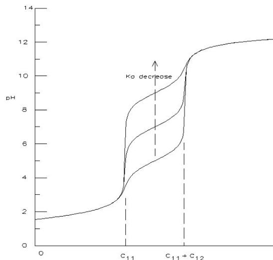
Fig. 3. Titration curves of the three parameter model.
