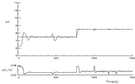
Fig. 11. Experimental results of the control system with three parameter model: run 1.
